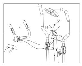
Remove four M5x12 Bolts (97) from the back of the Computer (96). Remove bolts with the Multi Hex Tool with Phillips Screwdriver provided.
