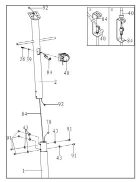
Remove six M8x15 Bolts (91), six Ø20xØ8x2.0 Big Curve Washers (43), from the Main Frame (1). Remove bolts and washers with the S6 Allen Wrench provided.
